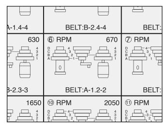
Figure 28. Pulley combination for 670 RPM for example.
